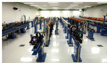
Laser amplifiers in the PALS laser hall
