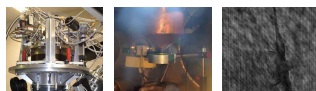
Helium cryostat (left) producing a thin band of H-ice (middle), and interferogram-shadowgram of the hydrogen plasma
